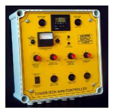
Provides TDS conductivity bleed control, Dual Biocide with 15-1 ratio facility, proportional inhibitor Dosing, 0-6 bleed lockout timer activated by either biocide pump.
